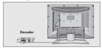
1 Connect the »AV1 « socket on the television set and the appropriate socket on the decoder using a EURO-AV cable.
